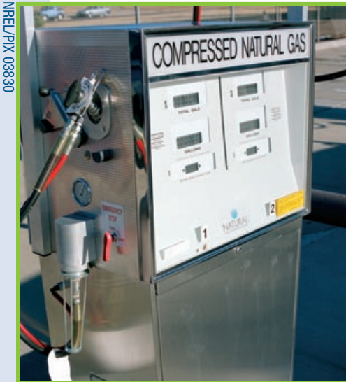
Fast-fill CNG pumps look much like a conventional gasoline pump. Fast-fill dispensers fuel CNG vehicles quickly.
