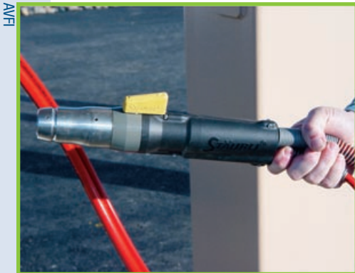
This Type 1 nozzle is typically what drivers will find at a public CNG fueling station.
