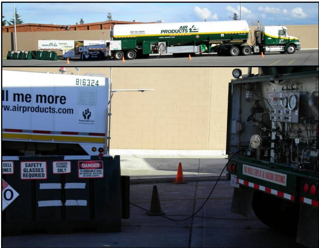
Figure 4. Tanker truck filling APCI mobile fueler (top) and up-close picture of the connection between the tanker and fueler (bottom)
