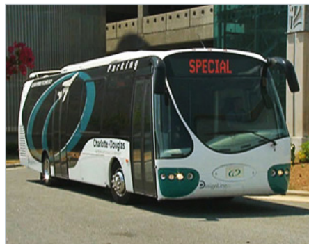
These 35-foot plug-in hybrid buses at Charlotte Douglas International Airport run in full-electric, zero-emissions mode over a third of the time. Photo from MotorWeek
