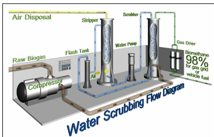
FIGURE 7 Schematic of Greenlane water scrubbing system (left panel; graphic courtesy of Greenlane Biogas, http://greenlanebiogas.co.uk/americas/greenlane-technology .); the Fair Oaks biogas upgrade plant (right panel; photo courtesy of DVO, Fair Oaks Dairies Gallery, http://www.dvoinc.com .)
