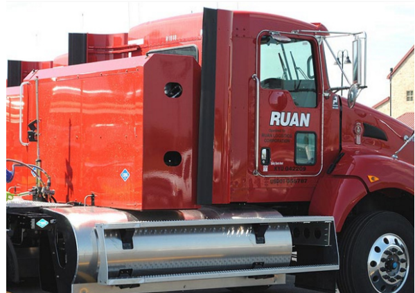
FIGURE 1 A truck in the Fair Oaks Dairy fleet, showing back-of-cab and saddle tanks. (Photo courtesy of ampCNG.)
