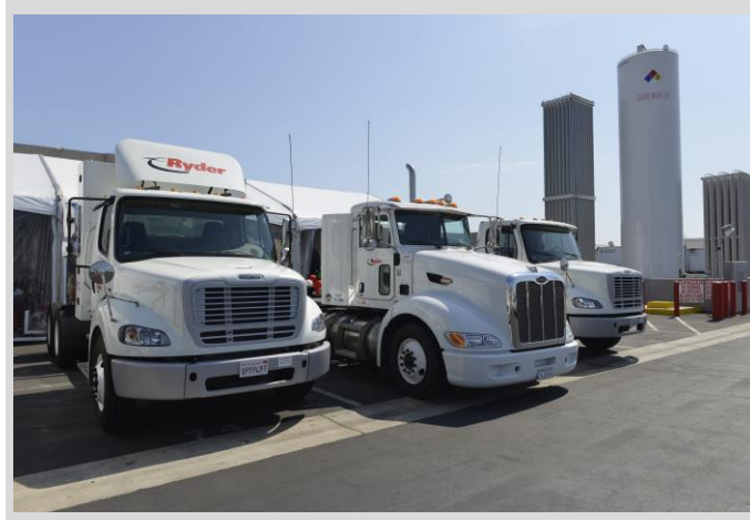
Figure 1. Ryder Natural Gas Trucks: Freightliner CNG (left), Peterbilt LNG (center), Freightliner LNG (right)
