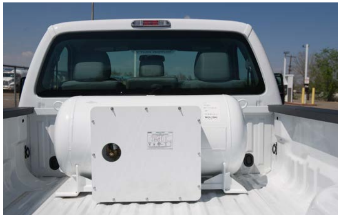
This Ford F250 pickup truck was converted to run on propane. Photo by Dennis Schroeder, NREL 33407
