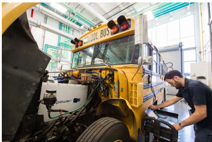
National Renewable Energy Laboratory researcher Andrew Meintz runs tests on a school bus that has been repowered with an electric motor. Photo by Dennis Schroeder, NREL 38951
