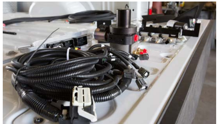
This kit allows a gasoline-powered vehicle to be converted to run on CNG. Photo by Amy Glickson, NREL 44909
