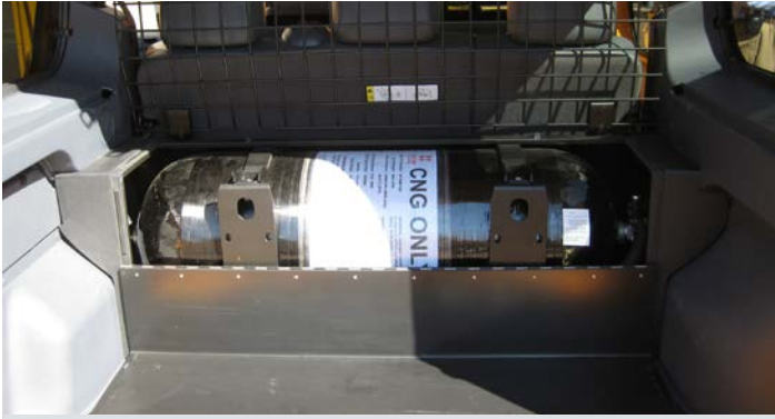
Depending on the application and installation, extra storage tanks may displace cargo capacity, as seen in this Ford Transit taxi (pictured with its protective tank cover open for demonstration purposes) that was converted to CNG. Photo by Margaret Smith, NREL 18210
