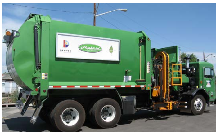
The City and County of Denver's vehicle fleet includes hydraulic hybrid refuse hauler trucks. This technology is ideal for stop-and-go trash collection operations. Photo from Denver Fleet Management, NREL 17153
