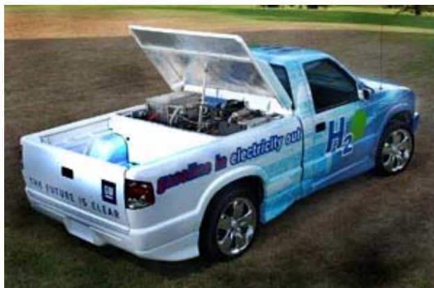
Chevrolet S-10 truck with on-board gasoline reformer.
