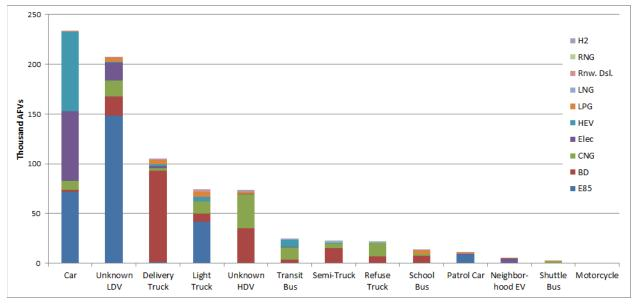
Figure 9. AFVs by vehicle and fuel type
