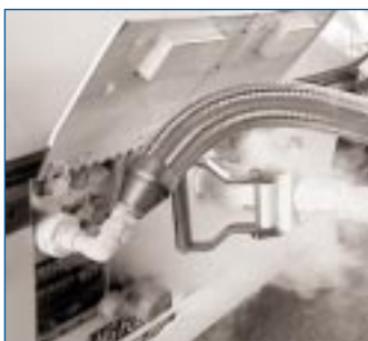
Figure 8. LNG fueling hoses connected to DART bus
