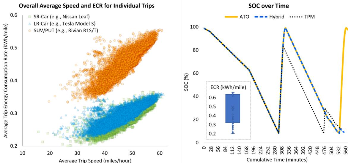
**Figure 7. (Left) ECR (kWh/mile) for each trip simulated in the spectrum of average trip speed. (Right) Example of the evolution of SOC throughout the trip, illustrating the three different charging behaviors evaluated: always topping off (ATO), time penalty minimization (TPM), and hybrid**
