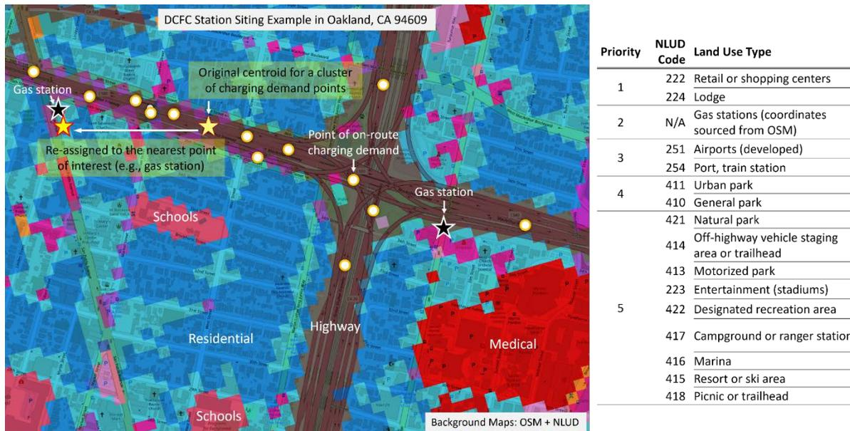
**Figure 8. (Left) An example of DCFC station siting—reassigning the centroid of a cluster of charging demand points along the road network to the nearest gas station (going with the second priority due to the lack of retail locations nearby). NLUD has a 30-m by 30-m resolution showing the representative land use type for each cell. (Right) List of ranked land use types and NLUD codes, including gas stations, based on OSM**
