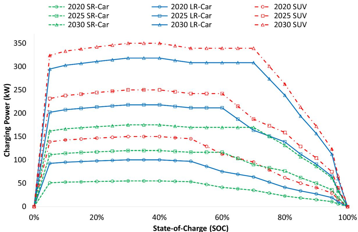
**Figure 5. The level of DCFC power that BEVs can accept at charging stations varies with vehicle type (e.g., long-range SUV vs. short-range small car), model year (2020 vs. 2030), etc.**
