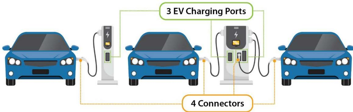
**Figure 9. An illustration of a charging station that has three charging ports and four connectors**
