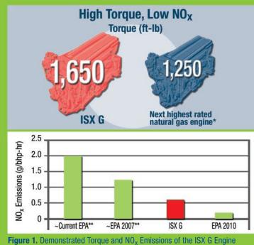
Figure 1. Demonstrated Torque and  $NO_x$  Emissions of the ISX G Engin Developed in this Project
