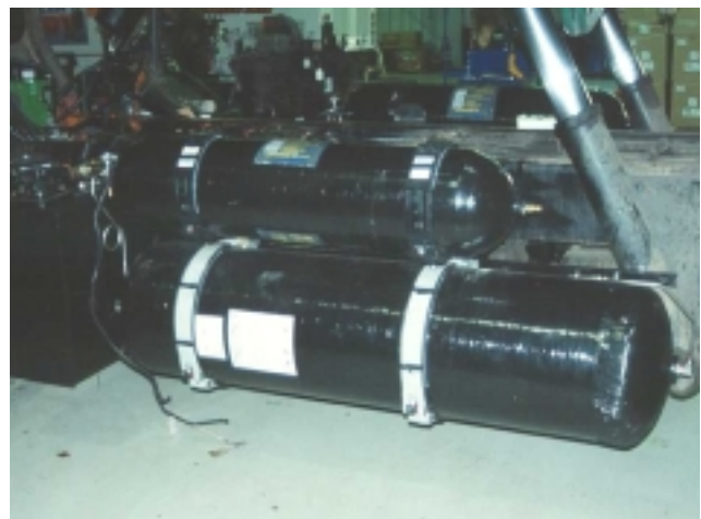
Photos 5-3 & 5-4. Left-hand and Right-hand Views of CNG Tanks Installed on the P320 Trash Truck Chassis Owned by WMI.
