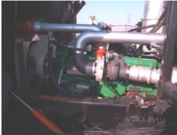
Photos 5-1 & 5-2. Left hand and Right hand Views of the John Deere 8.1L NG Engine in Chassis.
