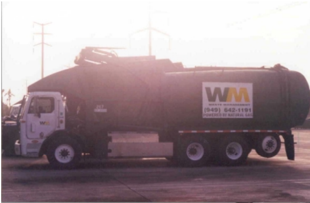
Photo 5-5. Left-hand View of WMI Trash Truck Following the Retrofit with a 280 HP John Deere 8.1L CNG Engine
