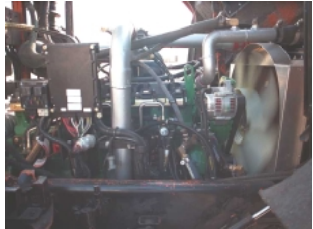
Photos 5-1 & 5-2. Left hand and Right hand Views of the John Deere 8.1L NG Engine in Chassis.
