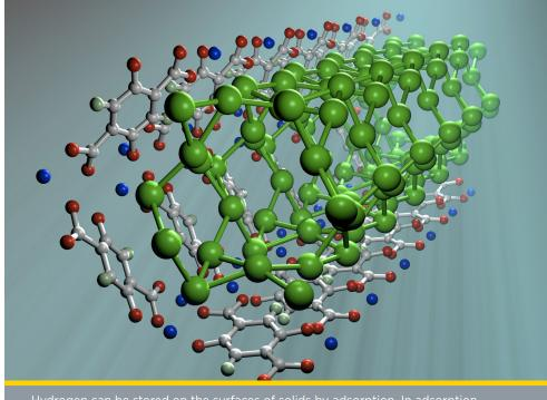
Hydrogen can be stored on the surfaces of solids by adsorption. In adsorption, hydrogen associates with the surface of a material either as hydrogen molecules (H<sub>2</sub>) or hydrogen atoms (H). This figure depicts hydrogen adsorption within MOF-74.
