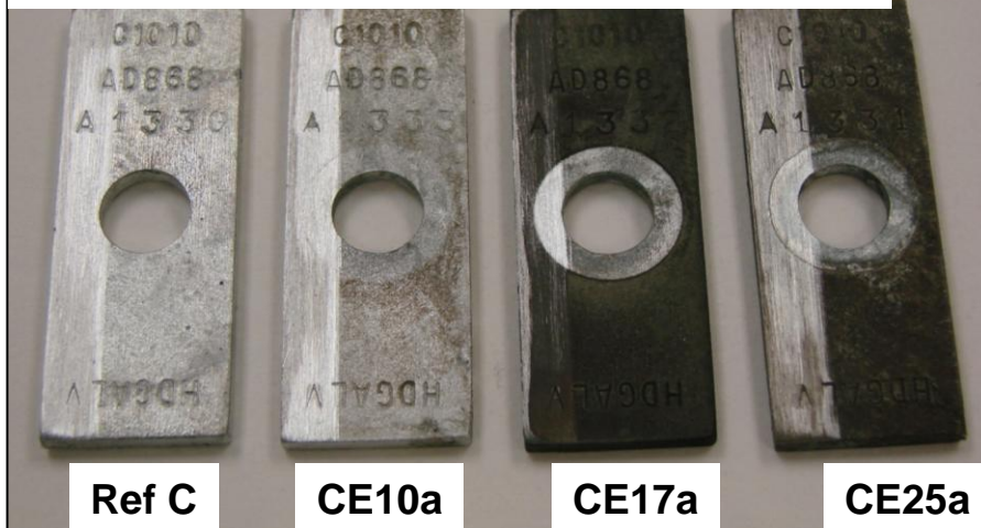
Zn-plated steel, substrate partially exposed
