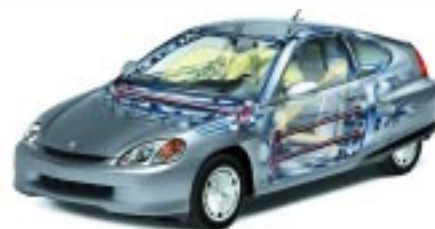
The body of the Insight is 40% lighter than those of comparable cars.
