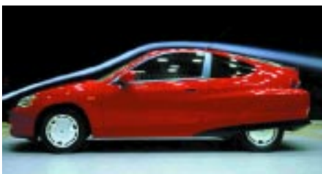
Aerodynamic features reduce drag.
