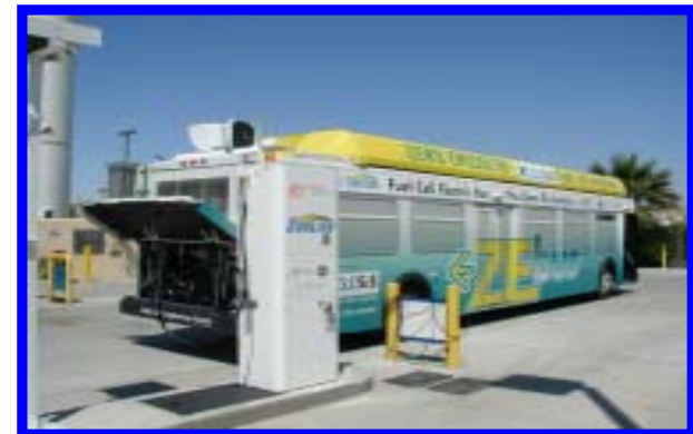
Ballard - Xcellsis demonstration bus powered by a hydrogen-fueled proton exchange membrane fuel cell, fueling at SunLine Transit Agency's solar hydrogen station
