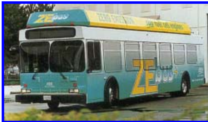
Ballard - Xcellsis demonstration bus powered by a hydrogen-fueled proton exchange membrane fuel cell, fueling at SunLine Transit Agency's solar hydrogen station
