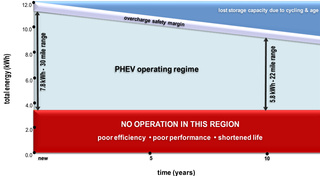
Figure 30: Potential battery pack conceptual design without reserve capacity to accommodate cycling and aging losses
