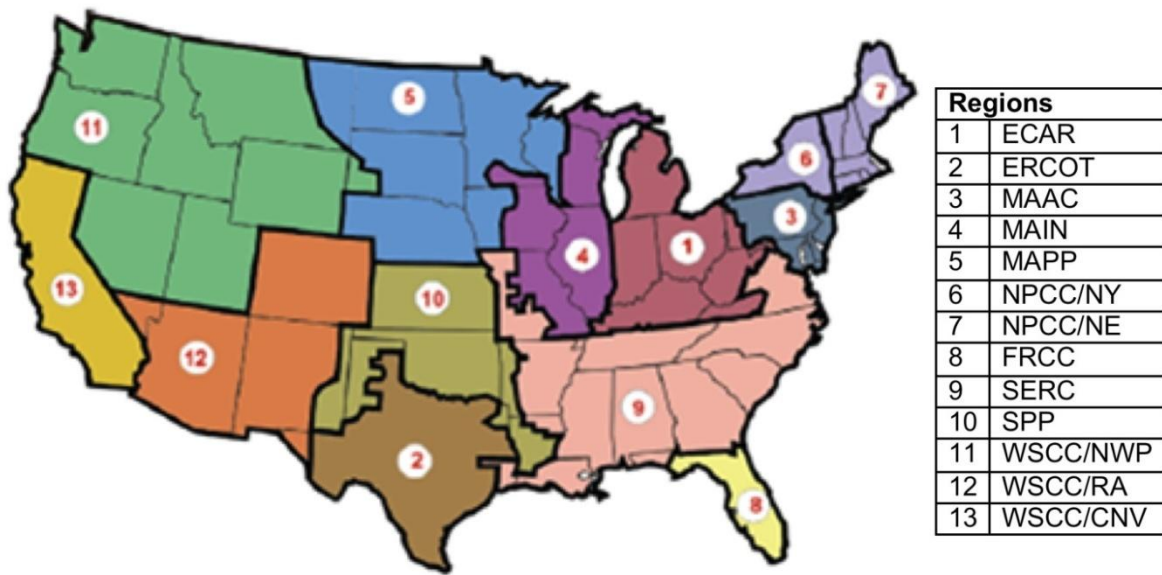
Figure C - 2: Thirteen NERC Regions, as of 2003, used in NEMS and other models. [Note: The ECAR region is no longer in operation.]
