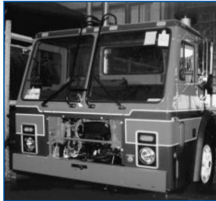
The first Mack LE refuse hauler being fitted with the natural gas E7 engine
