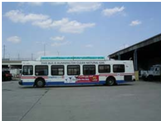
Figure 4: MY 2001 New Flyer C40LF Bus with MY 2001 CWI C Gas Plus CNG Engine
