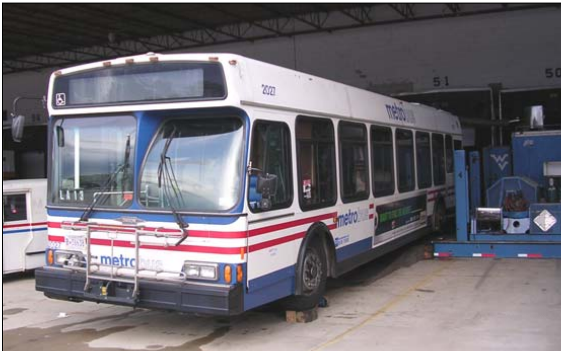
Figure 6: Bus under Test on the WVU TransLab Chassis Dynamometer
