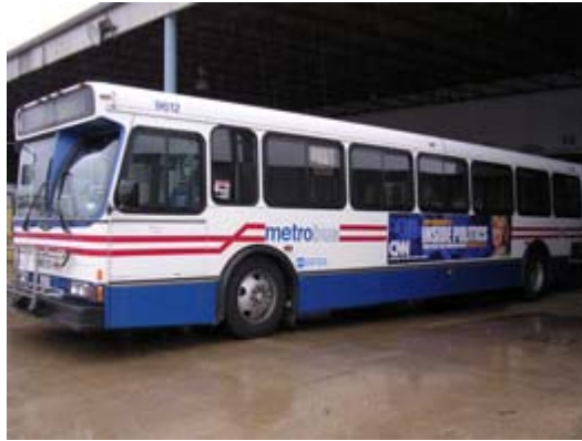
Figure 3: MY 1992 Orion Model 06.501 Bus with MY 2004 DDC Series 50 Engine and EGR
