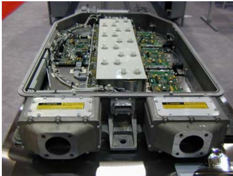
Figure 9. Dual-Power Inverter Module
