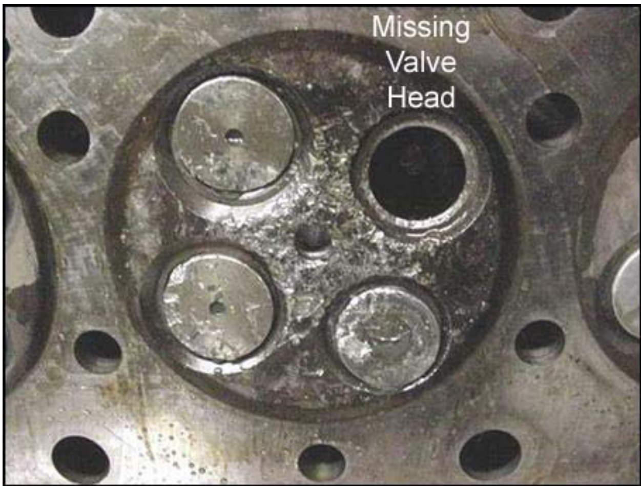
Figure 12. Broken Intake Valve Head on Cylinder 3
