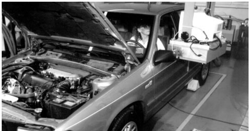
This light-duty vehicle undergoes an FTP emissions test on a chassis dynamometer at Mantech.
