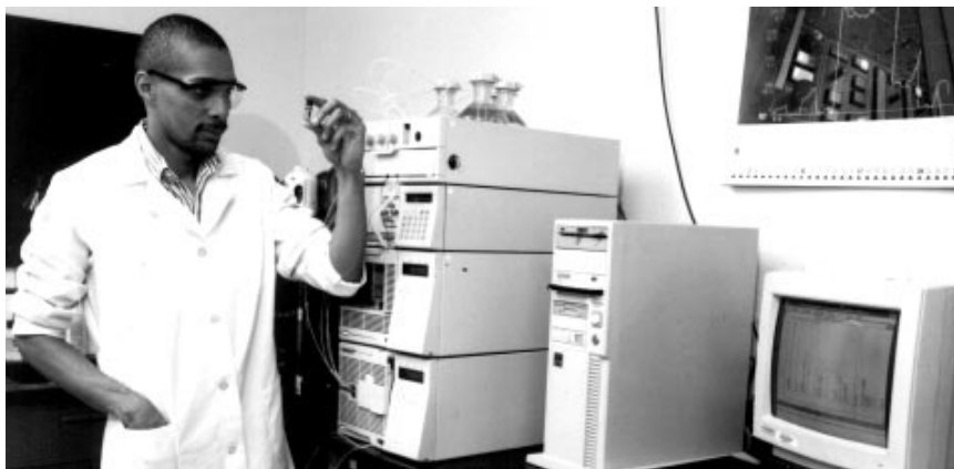
A technician from Mantech Environmental Technology of Denver, Colorado, analyzes aldehyde emissions with a liquid chromatograph.
