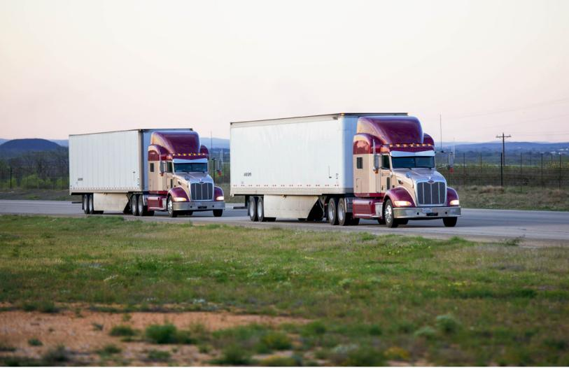
NREL researchers are evaluating truck platooning, a strategy to reduce aerodynamic drag by grouping tractor trailers closely together on the highway. Photo from Peloton, NREL 31237
