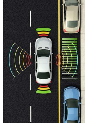
Automated vehicles use computer algorithms, sensors, and cameras to navigate the road without human assistance. Many models today offer semi-automated capabilities, such as parallel-parking assistance. Photo from iStock, 20606281
