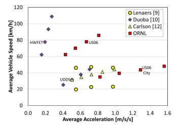
Figure 23. Comparison of drive cycles using average vehicle speed and average acceleration as metrics.
