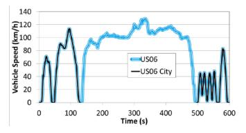
Figure 12. The US06 City cycle is represented by the two portions of the US06 trace shown in black. The US06 City cycle retains much of the hard accelerations and decelerations of the US06.
