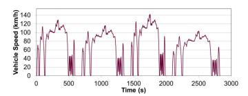
Figure 16. US06-based cycles are shown in the experimental sequence used for the conventional vehicle with intensity scaling factors of 1.0, 0.9, 1.1, and 0.8, respectively.
