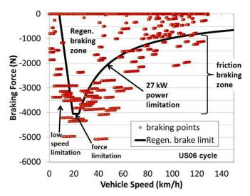
Figure 9. RB limits for a 2011 Sonata HEV and calculated brake force needed over the US06 cycle.
