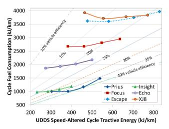
Figure 25. Fuel energy as a function of tractive energy for six vehicles for speed multiplied UDDS cycles in [10] (speed multipliers are 0.8, 1.0, 1.2, and 1.4).
