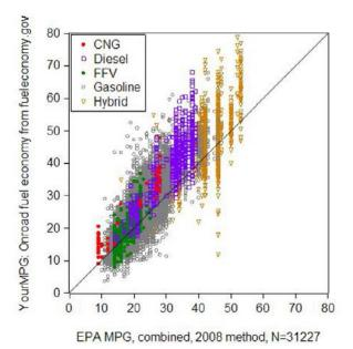
Figure 1. Self-reported miles per gallon (mpg) values from <u>www.</u> <u>fueleconomy.gov</u> plotted against the EPA label values. CNG = compressed natural gas; FFV = Flexible Fuel Vehicle
