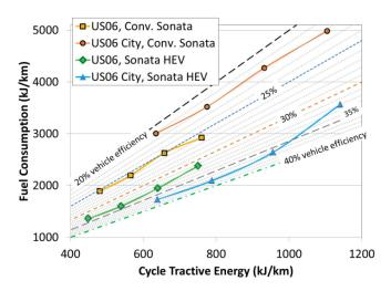
Figure 24. Fuel energy as a function of tractive energy for the conventional and hybrid Hyundai Sonatas over intensity modified US06 and US06 City cycles.
