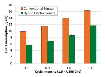
Figure 19. Experimental FC results for the conventional and hybrid Hyundai Sonatas as a function of US06 City-based cycles with altered intensity levels.
