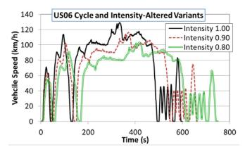
Figure 11. The US06 cycle can be modified in intensity to form variants with lower or higher speeds and rates of accelerations and decelerations.
