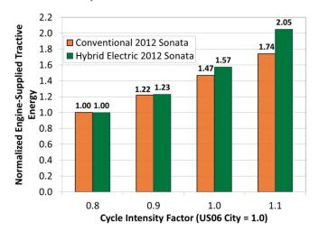
Figure 15. Normalized engine-supplied tractive energy as a function of US06 City-based drive cycle.
