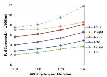
Figure 5. Results for FC for six vehicles tested over the HWFET cycle and intensity variant cycles altered by speed multipliers [10].
