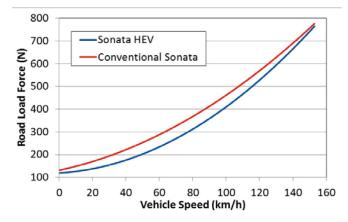
Figure 10. Road-load force curves for the 2011 Hyundai Sonata hybrid and conventional vehicles.
