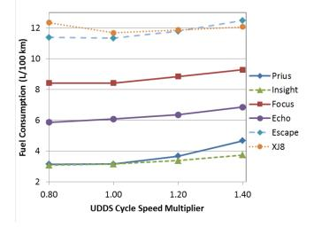
Figure 4. Results for FC for six vehicles tested over the UDDS cycle and intensity variant cycles altered by speed multipliers [10].
