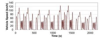
Figure 17. US06 City-based cycles are shown in the experimental sequence used for the conventional vehicle with intensity scaling factors of 1.0, 0.9, 1.1, and 0.8, respectively. The sequence features pairs of identical cycles to create a longer drive length for each condition.
