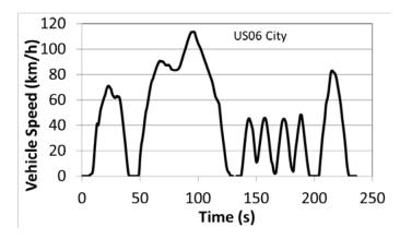
Figure 13. The US06 City cycle is shown here as one continuous cycle.
