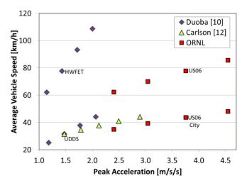
Figure 22. Comparison of studied drive cycles using average vehicle speed and maximum acceleration as metrics.
