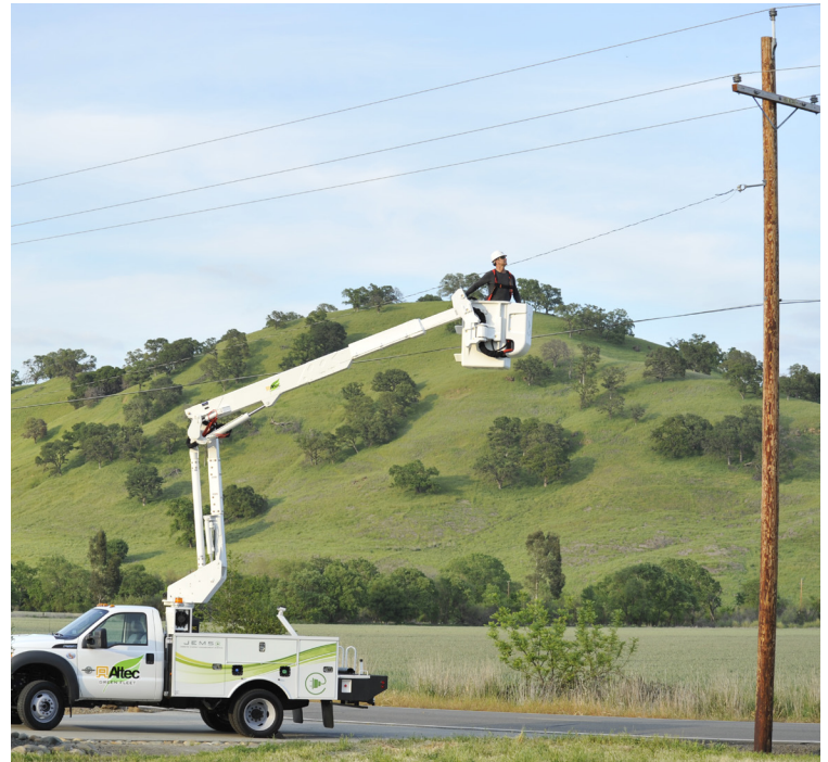
Hybrid utility truck allows for work on utility lines without engine idling. Photo credit: Altec, Inc.
