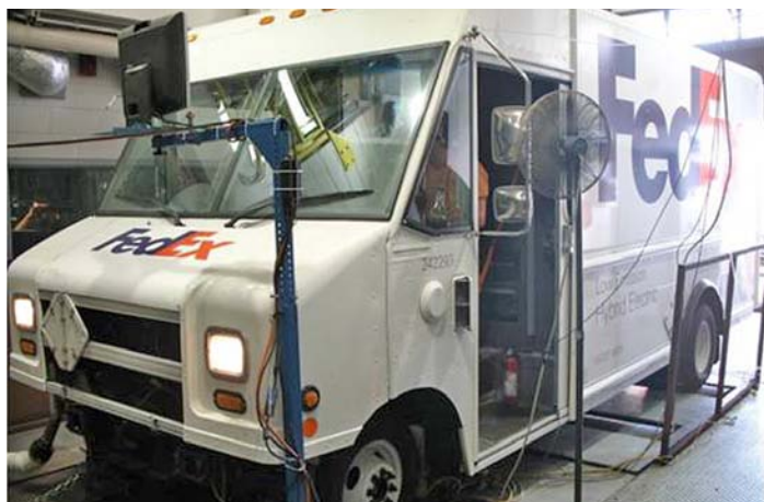
Fleet vehicle on the chassis dynamometer. Photo by Scott Walters, NREL/PIX 19908
