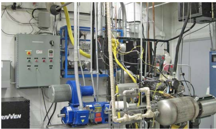
Light-duty engine dynamometer test cell. Photo by Xin He, NREL/PIX 19907
