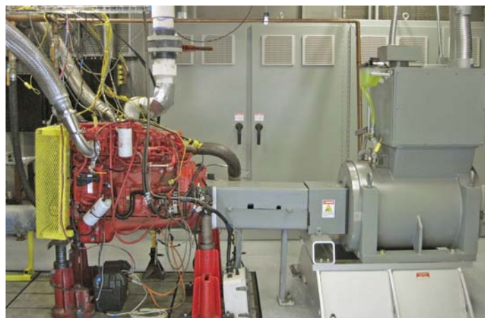
Heavy-duty engine dynamometer test cell. Photo by Matthew Thornton, NREL/PIX 19906
